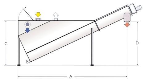
Outlet side is optional – a blinding flange is supplied with the machine
