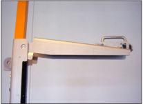
Locking device which can be folded under walking area.
