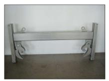
Lifting tool. By using sectional Stop Logs and our specially designed lifting
