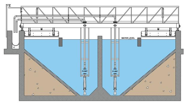
The grit and grease travelling bridge KD 22 consists of a complete travelling bridge with separate drive unit, mechanical surface scrapers for collection of surface sediment and submersible pump unit (optional) for collection of settled grit.
