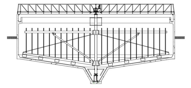
The functioning of the sludge thickener is to convey the sludge from bio-tanks etc. to the storage tank, which comprises a slow-acting agitator having a bottom scraper (leading the thickened sludge to a centre pit, vertical bars for the gentle stirring of the sludge and at the same time assuring the necessary passage for the capillary water to reach the surface).
