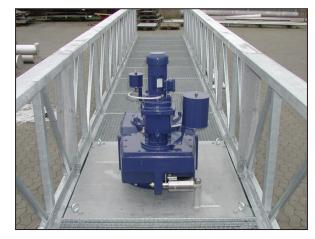
and the thickened sludge is discharged through the bottom "sludge pit", the reject water "the capillary water" is removed in an overflow spout, placed at the lateral faces of the container.
