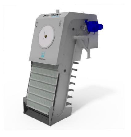
The KD43 band screen ensures effective fine screening and separation of grit in wastewater. KD's unique band screen is the only one on the market where the screen plates open at the back on the way down. This gives a significantly lower pressure drop than a traditional band screen, and at the same time accumulation of grit inside the
